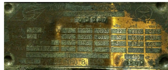
FIGURE 5. eHPCC – Electric motor nameplate.
