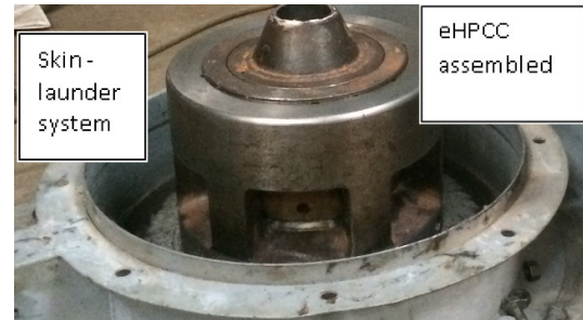
FIGURE 3. Laboratory-scale eHPCC without top skin showing the launder system.
